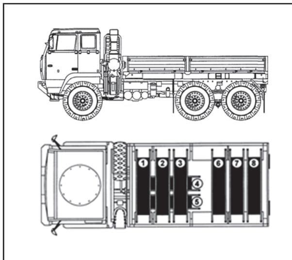
**Figure 3-3. Loading the M1093, MTV, 5 ton**
