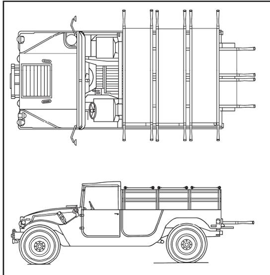
**Figure 3-2. M998 truck, cargo/troop carrier 1 1/4 ton, HMMWV (two-man configuration), with five litters**
