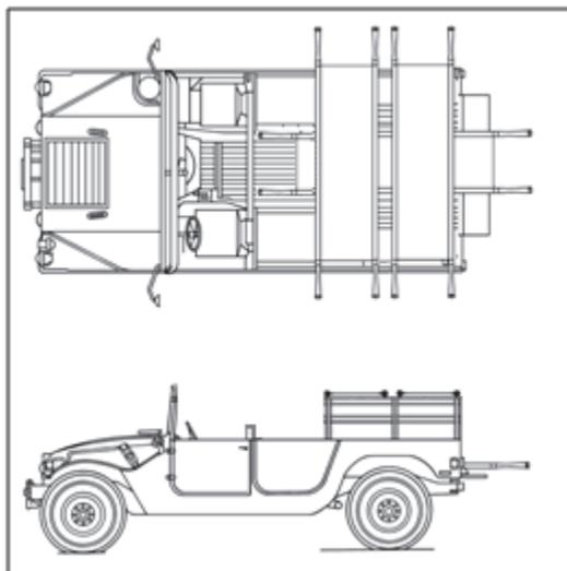
**Figure 3-1. M998 truck, cargo/troop carrier 1 1/4 ton, HMMWV (four-man configuration), with three litters**
