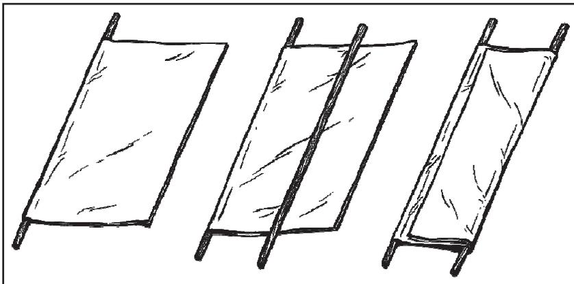
Figure 2-14. Litter made with blankets and poles
