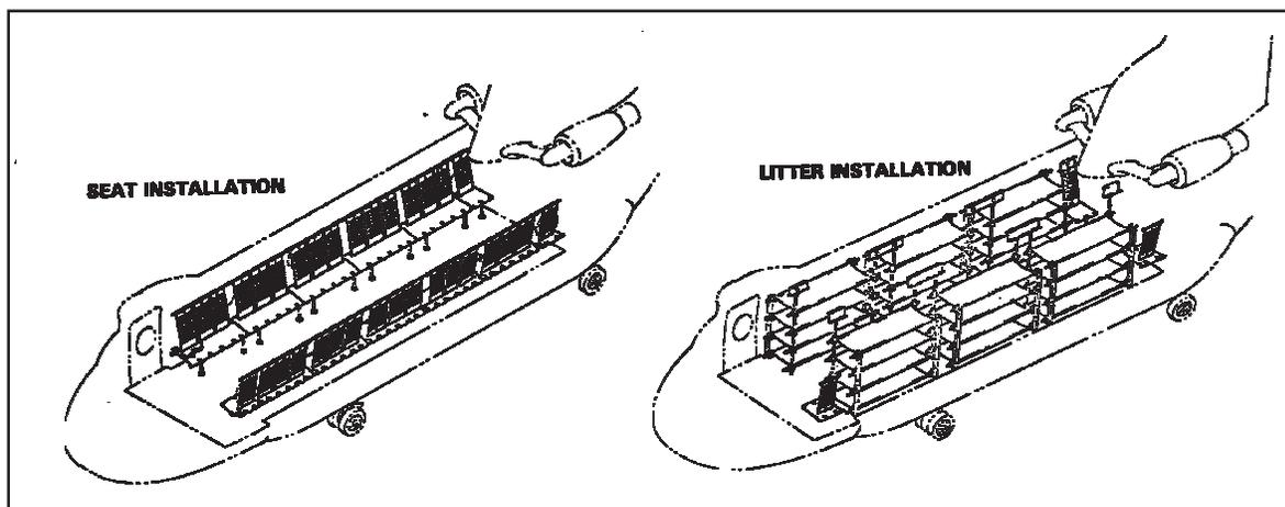
Figure 3-8. Interior view of CH-47 (Chinook) with litter installation
