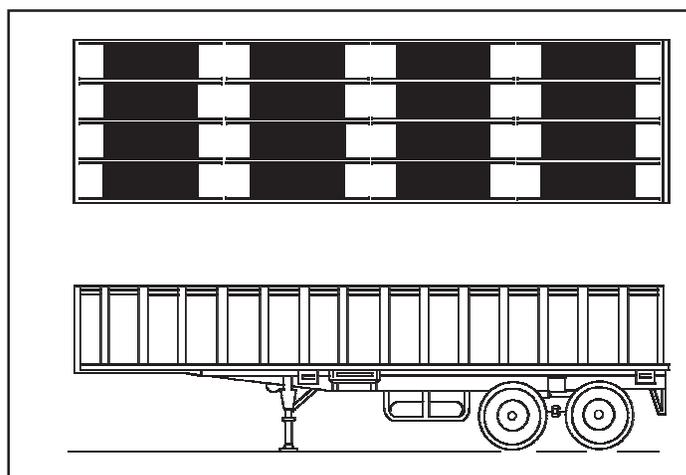
**Figure 3-6. M871 22 1/2 ton, cargo semitrailer, loaded with litters**
