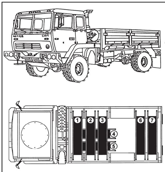
**Figure 3-4. Loading the M1081, LMTV, 2 1/2 ton**
